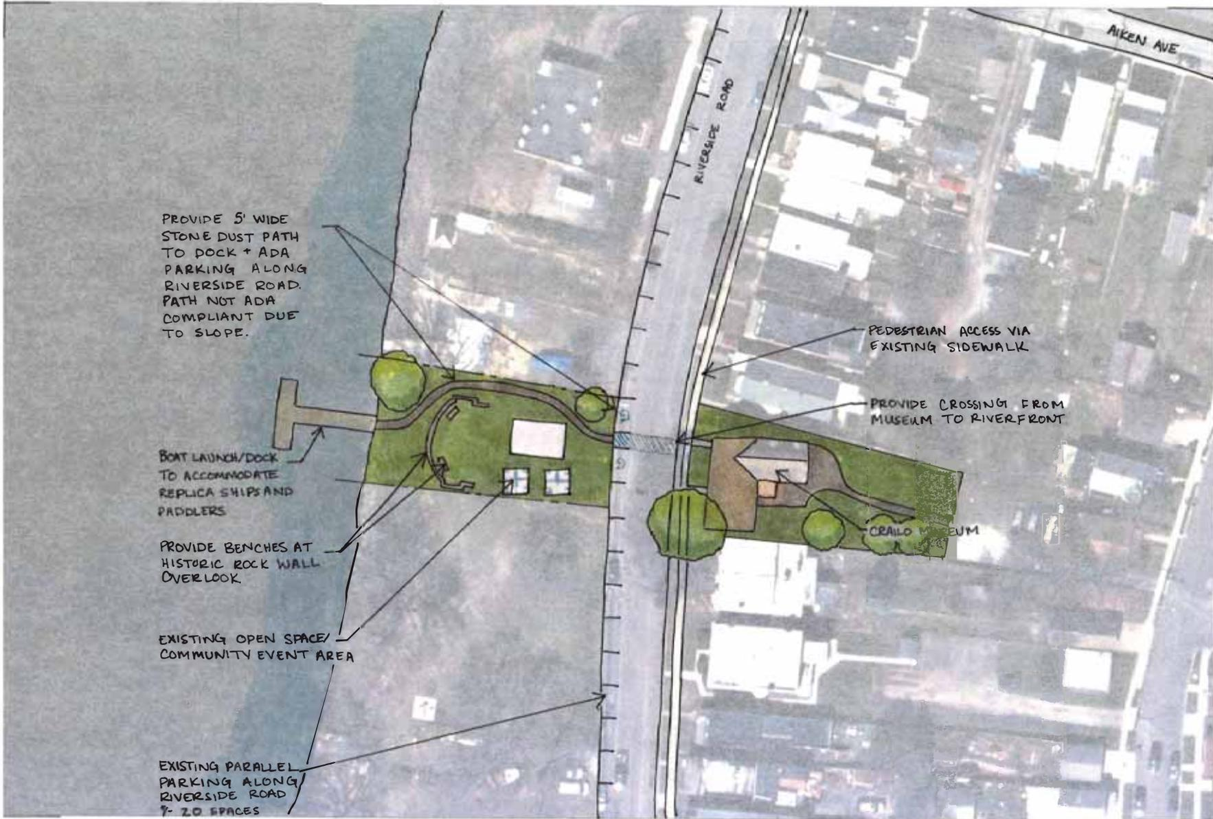
PROVIDE 5' WIDE STONE DUST PATH TO DOCK + ADA PARKING ALONG RIVERSIDE ROAD. PATH NOT ADA COMPLIANT DUE TO SLOPE.
